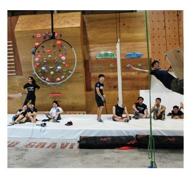
Permanent cover boulder mats are design in one piece cover over the whole area which is the most durable landing solution for large areas. the flooring is non-movable, and requires and experience crew for onsite installation. The mat id fixed to the floor with seamless joining to prevent displacement of the mat and are estetically pleasing
